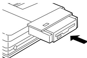
Insert an MP unit into the slot.
