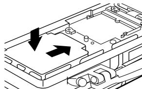
Slide the battery pack inward until it is firmly in place.
