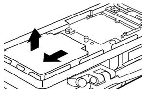
Slide the battery pack toward the outside edge to remove it.
