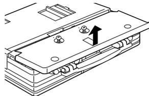
Use a screwdriver to loosen the two screws located toward the front of the computer.
