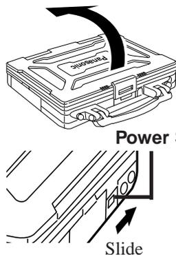
Lift the latch and open up the display.
