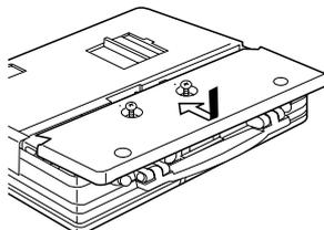
Replace the cover and tighten the two screws.
