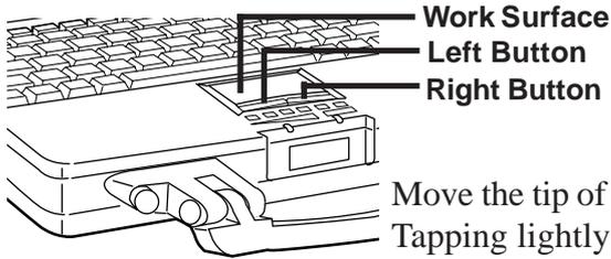
Move the tip of your finger lightly over the surface to move the cursor. Tapping lightly on the surface has the same effect as clicking the left mouse button.
